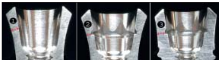
Fig 1 Cross section of 3 implant neck designs. The following are the indicated wall dimensions for the standard 4.1 ( left ), synOcta 4.1 ( middle ), and synOcta TE ( right ) implants, respectively, as reported by Straumann: 0.49 mm, 0.32 mm, and 0.53 mm.
