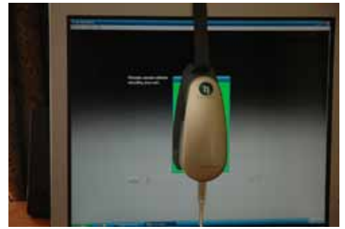
Figure 15 Calibrating both the laboratory and clinician's monitors with a spectrometer is critical for all subsequent color correction.
